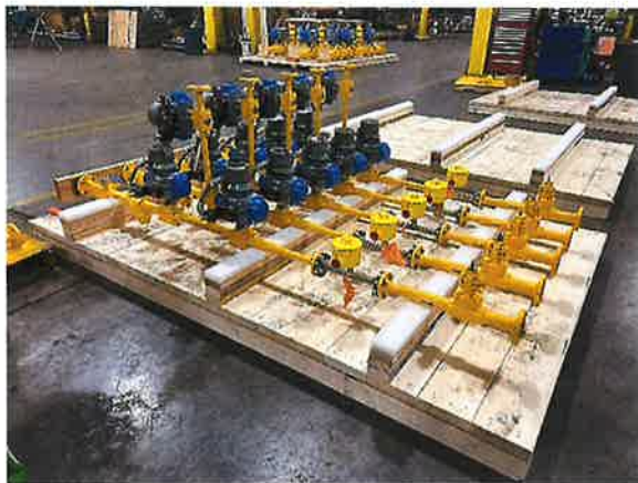
Natural Gas Burner Piping for a Coal Boiler conversion
