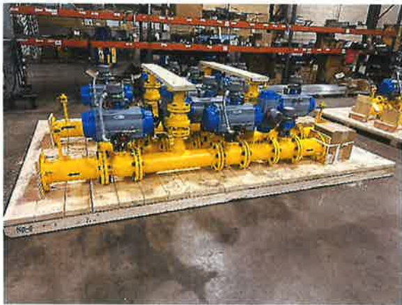
Natural Gas Burner Piping for a Coal Boiler conversion
